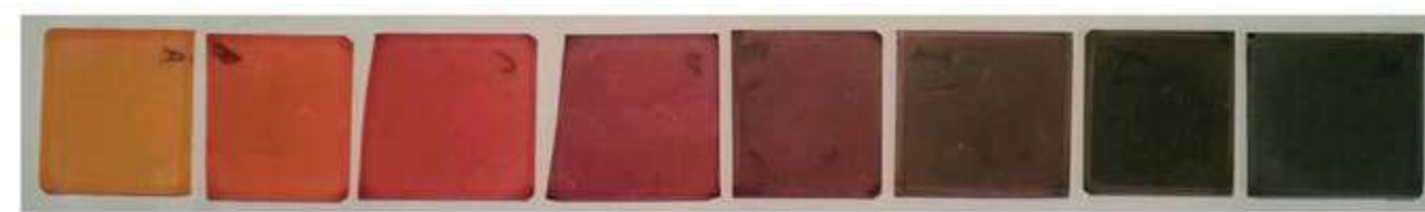
Fig. 2. Band gap engineering of perovskite (FAPbI 3 /Br 3-y ) films with different y values [5]
