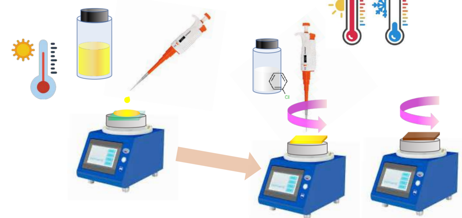
Fig. 7. Deposition of perovskite layers with different washing temperatures.
