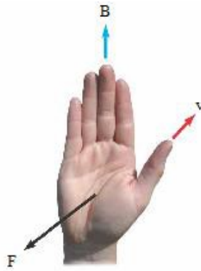
Figure 2. Right-hand rule; the vector \vec{v} is in the direction of your thumb and \vec{B} in the direction of your fingers. The force \vec{F}_B on a positive charge is in the direction of your palm, as if you are pushing the particle with your hand.
