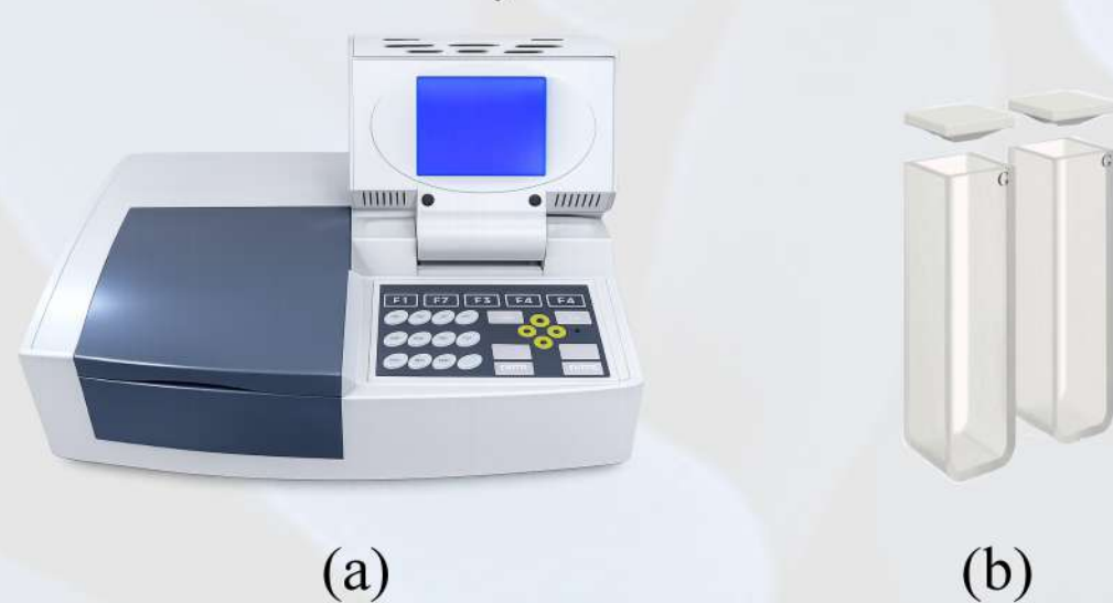
Figure 3: (a) UV-Vis spectrophotometer used for absorbance measurements of probiotic samples. (b) Quartz cuvettes used for spectrophotometric measurements.
