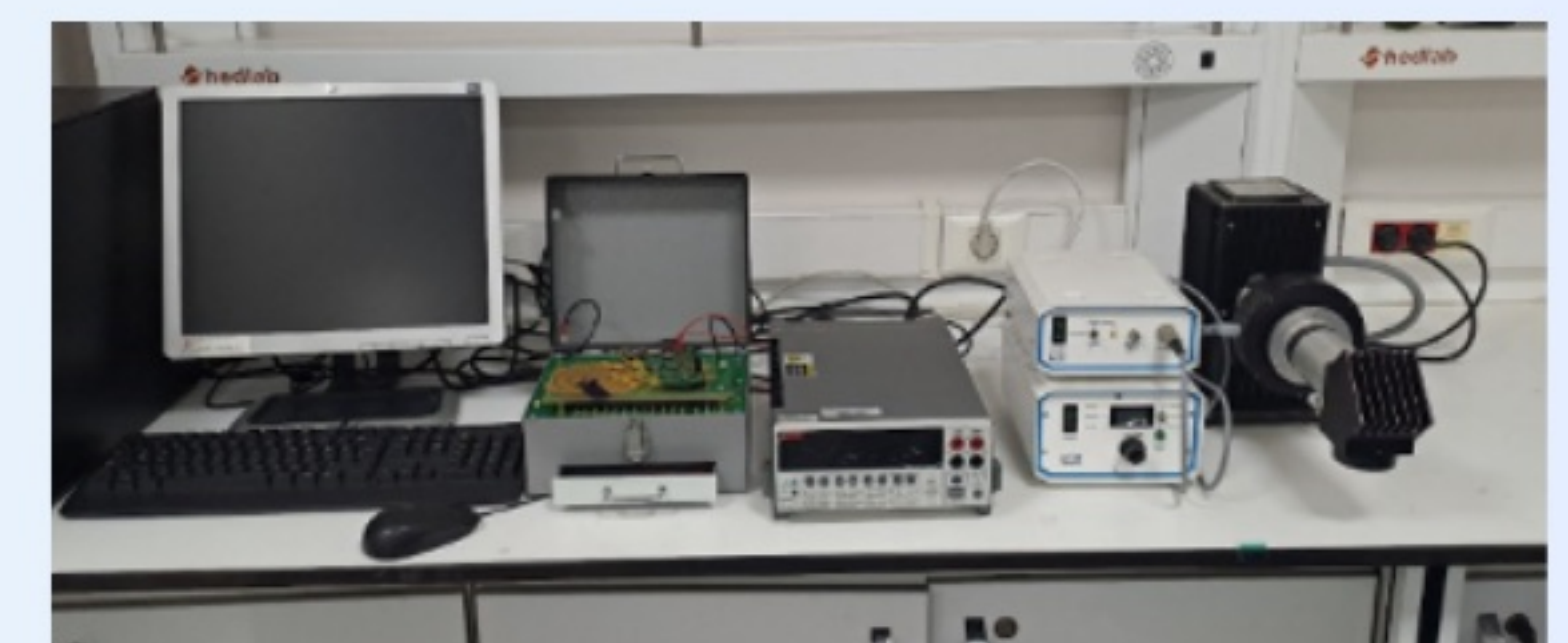
Figure 7.2: Experimental setup used for current-voltage (I-V) characterization.
