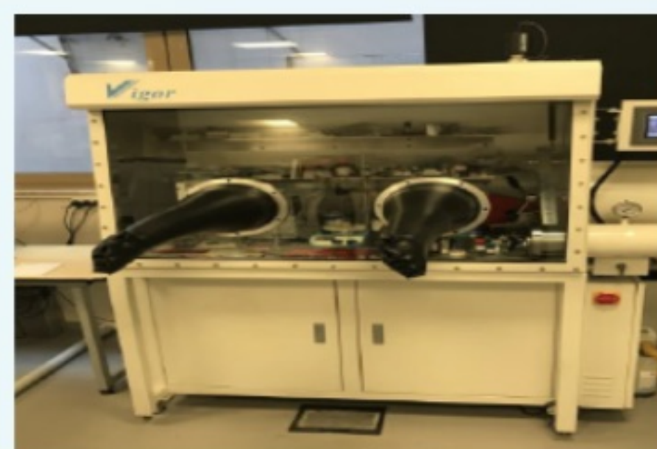
Figure 7.1: Nitrogen-filled glovebox system used for perovskite solution preparation, thin-film deposition, and electrical characterization under inert atmosphere to minimize moisture and oxygen-induced degradation.
