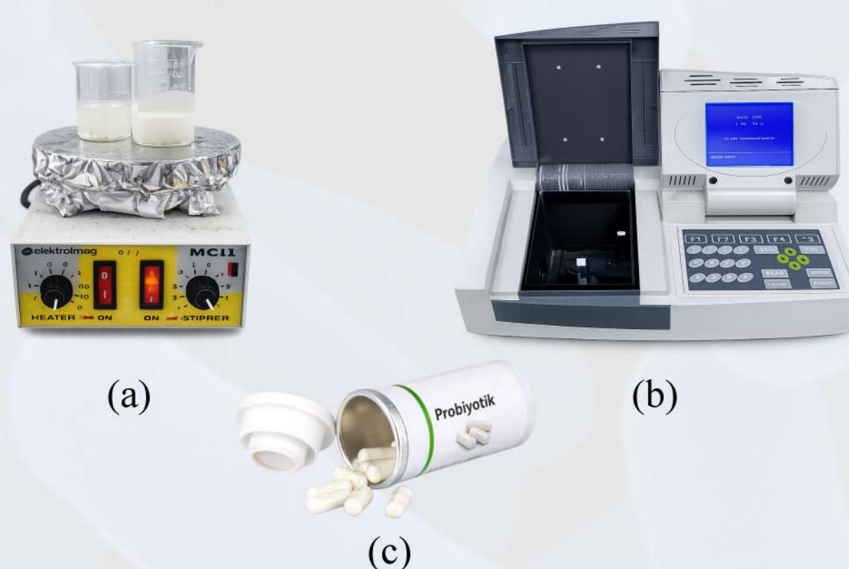
Figure 4: (a) magnetic stirring, (b) UV-Vis measurement. (c) probiotic capsule content after preparation.
