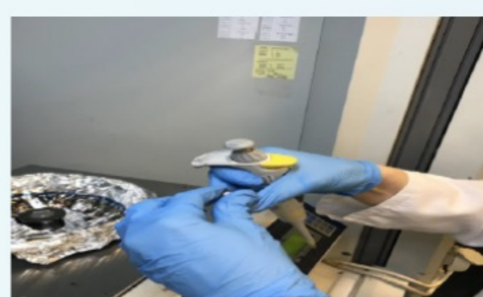
Figure 7.3: Spin-coating system used for the deposition of perovskite thin films during the preparation of the active layer in perovskite-based betavoltaic devices.
