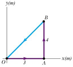
4) A force  $\vec{F} = (4x\hat{i} + 3y\hat{j})N$  acts on a particle as the object moves in the *x* direction from the origin to x = 5m. Find the work done on the object by the force.
